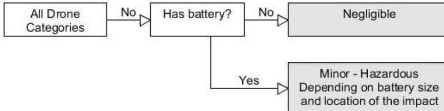
**Figure 7: Severity assessment in case of a drone collision when the drone has a battery.**
