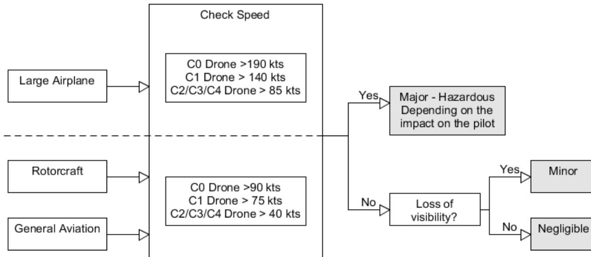
**Figure 11: Severity assessment in case of a drone collision which hits the aircraft's windshield.**
