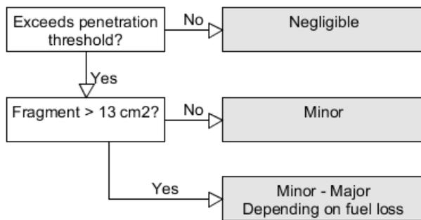
**Figure 9: Severity assessment in case of a drone collision which hits the aircraft’s fuel tank. Adapted from (Wilde & Draper, 2010)**
