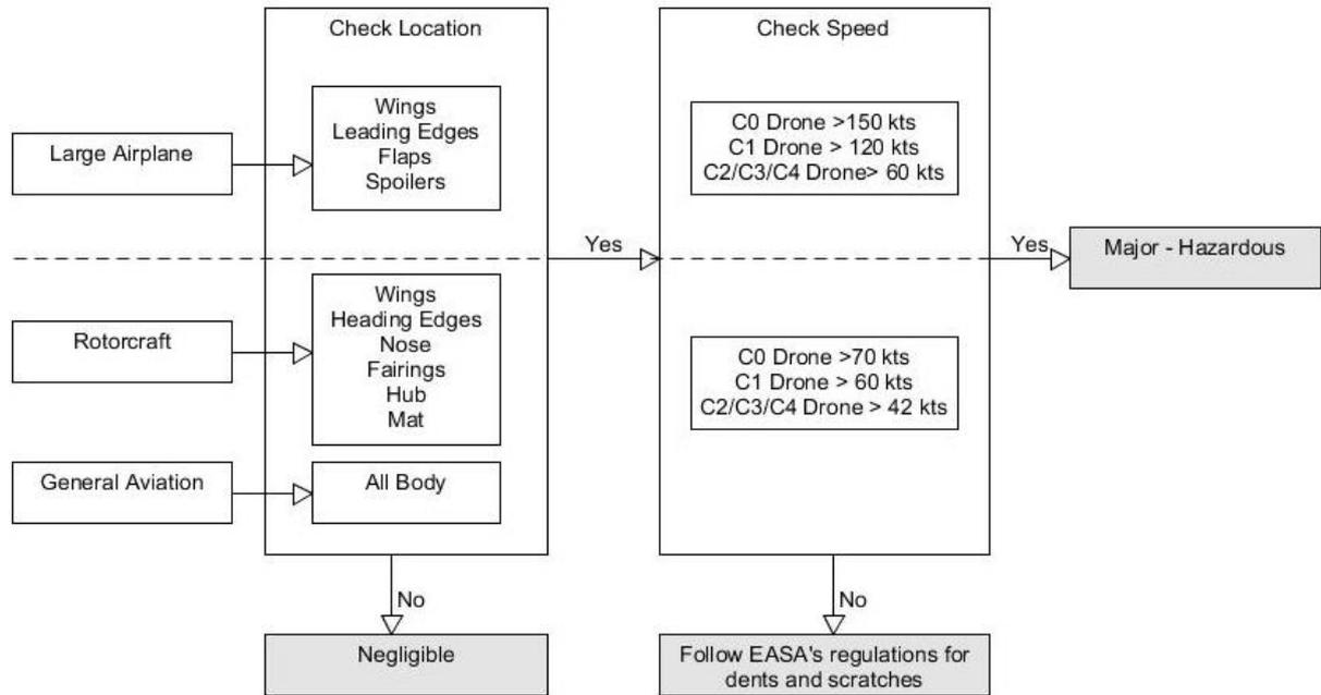
**Figure 10: Severity assessment in case of a drone collision which hits the aircraft fuselage.**
