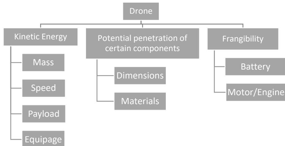
**Figure 6: Simplified model of a drone collision severity taxonomy. Adapted from (EASA, "Drone Collision" Task Force, 2016) and (FAA, FAA UAS Center of Excellence Task A4: UAS Ground Collision Severity Evaluation, 2017).**
