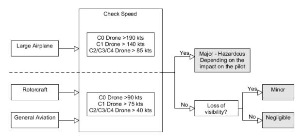
Figure 11: Severity assessment in case of a drone collision which hits the aircraft's windshield.
