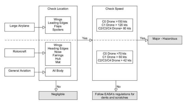
Figure 10: Severity assessment in case of a drone collision which hits the aircraft fuselage.
