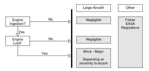
Figure 8: Severity assessment in case of a drone collision which hits the aircraft's engine.
