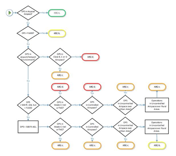
defined as "a qualitative classification of the rate at which a UAS would encounter a manned aircraft in typical generalized civil airspace"
