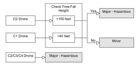
Figure 13: Severity assessment in case of a drone collision with a person. Adapted from (Shelley, 2016).
