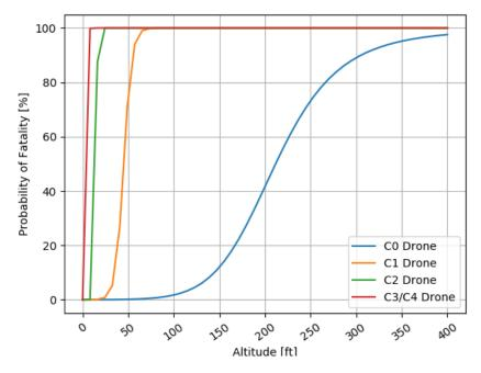
Figure 12: Probability of a Fatality if Impact Occurs, by type of drone and free fall height. Adapted from (Shelley, 2016).
