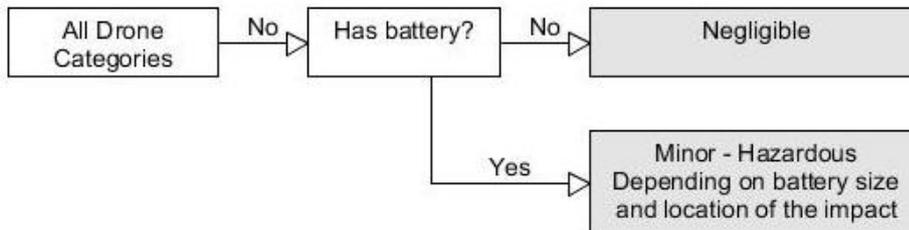
**Figure 7: Severity assessment in case of a drone collision when the drone has a battery.**
